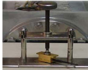
Test Sequence: After positioning the device, the puncture pin is driven through the package lid. The gas contained in the cavity then flows into the system for analysis.
