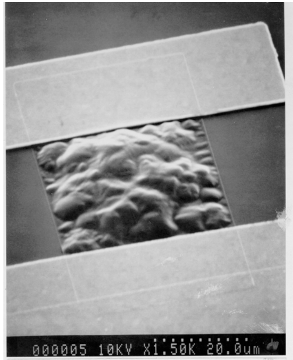
Figure 2, SEM at 1500X showing Titanium resistor forming the hydride.
